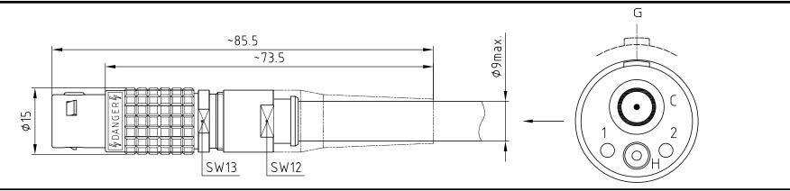
Outer shell Latch sleeve Collet nut Insulators Male contact (LV) Female contact (HV) Other metallic parts Heat shrink tubing
